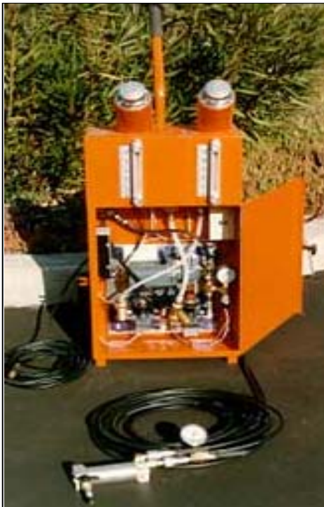
Example of an epoxy injection pump with a maximum delivery pressure of 200 psi. Pump is also designed to shut down if material ratios are incorrect or set pressures are exceeded.
